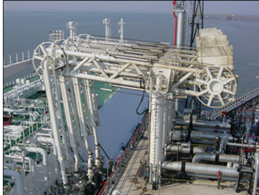
Figure 3: Sample of chiksan loading arms for LNG. Photo courtesy of FMC Technologies.
