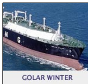
Figure 4: The Golar Winter , which uses a gas-transport membrane containment system built by Hyundai Heavy Industries is being converted to an FSRU and then leased to Petrobras for service at Guanabara Bay. Photo courtesy of Golar LNG.
